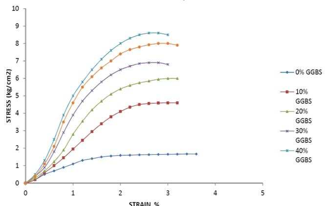
Fig.4. Stress-Strain behaviour of BC soil treated with GGBS for a curing period of 28 days
