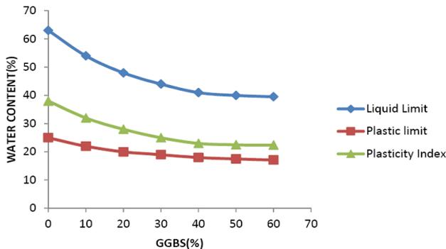
Fig. 1. Variations of liquid limit, plastic limit and plasticity index with addition of GGBS
