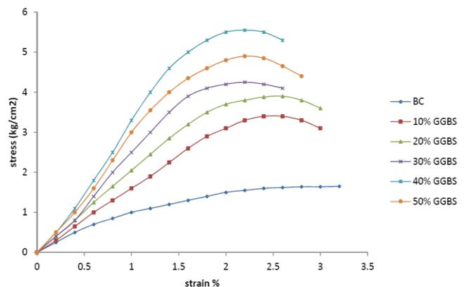
Fig.3. Stress-Strain behaviour of BC soil treated with GGBS for a curing period of 7 days
