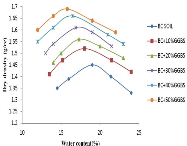
Fig.2. Variation of OMC vs. MDD with addition of GGBS to BC soil.
