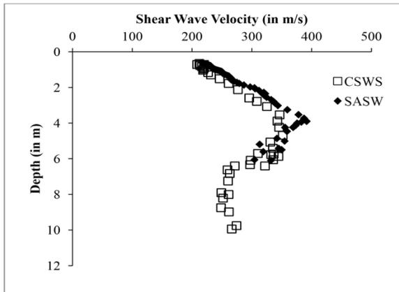
**Fig. 3.3** Variation of Shear Wave Velocity with Depth at St. Agnes School
