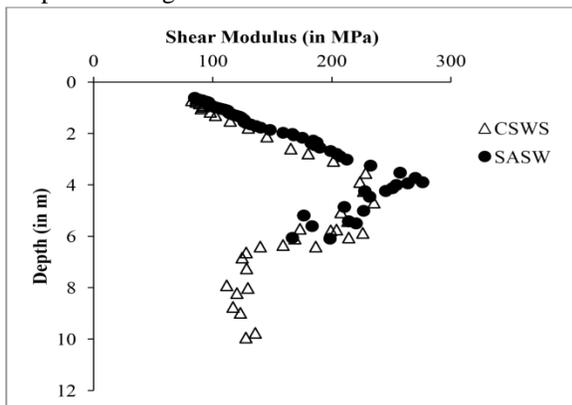
**Fig. 3.4** Variation of Shear Modulus with Depth at St. Agnes School
