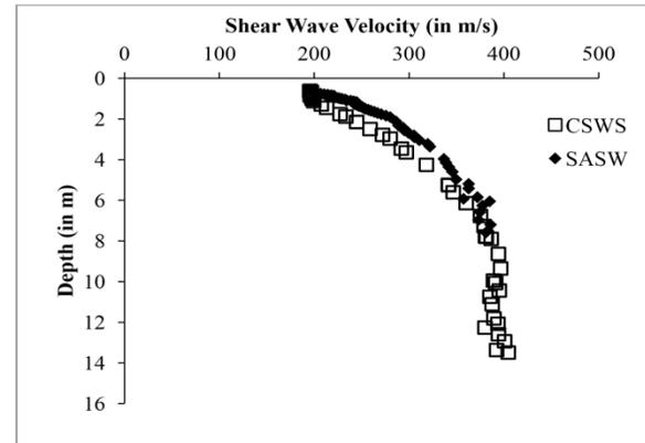
**Fig. 3.1** Variation of Shear Wave Velocity with Depth at Tata Sports Complex
