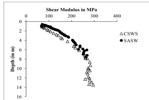
**Fig. 3.2** Variation of Shear Modulus with Depth at Tata Sports complex
