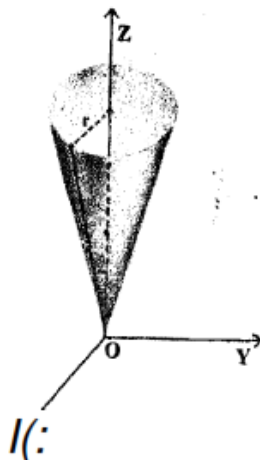
Fig. 4: A right circular cone with vertex at the origin and base curve x^2 + y^2 = r^2, z = k .
