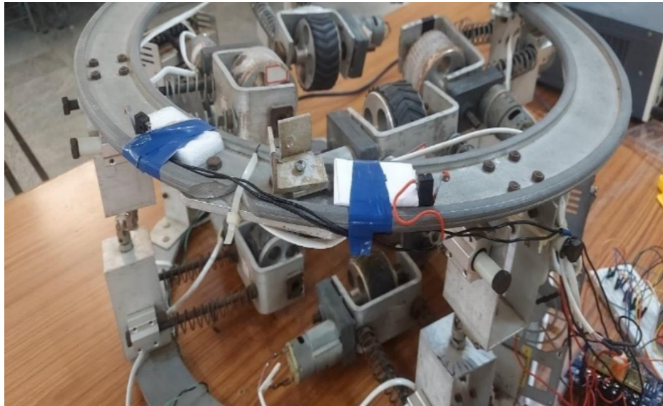
Fig 7.3: Installation of limit switches
