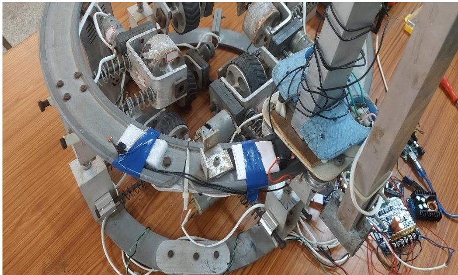
Fig 7.4: Controlling the Arm base motors with Limit Switches
