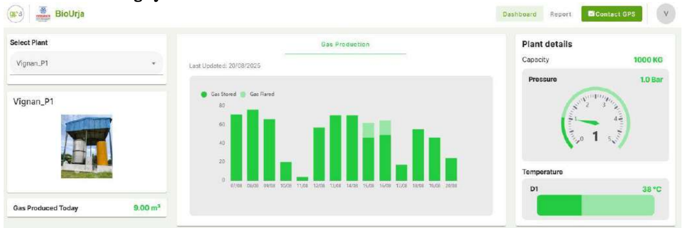
Figure showing Dashboard of Remote Monitoring System for BioUrja1000KPD
