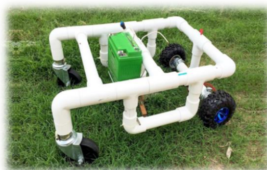
Remote controlled grass cutting machine
