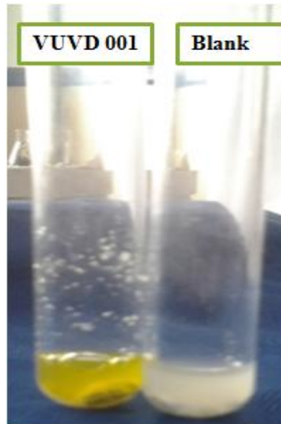
Fig. 3.6 Primary screening of lactase producing activity of VUVD001 by ONPG disc method
